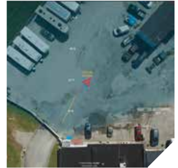
Security radar directs camera to track a vehicle on premise traveling 9.4 mph.
