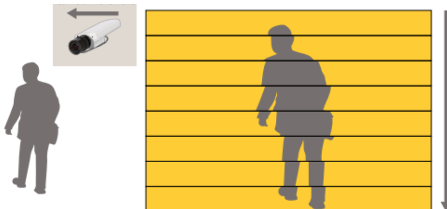
Figure 2. The principle of rolling shutter distortion. Lines are read out from the sensor from the top to the bottom of the image. When vibration is causing the camera to move slightly to the left while the lines are being read out, the result is a warped image.
