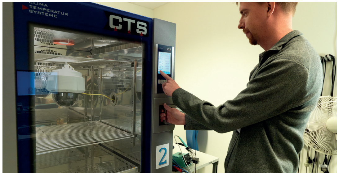
Figure 5: Temperature test in a climate chamber.
