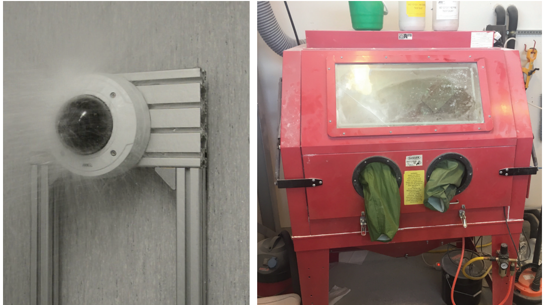
Figure 3: Left: Water-proof test of a camera, right: Dust lab.
