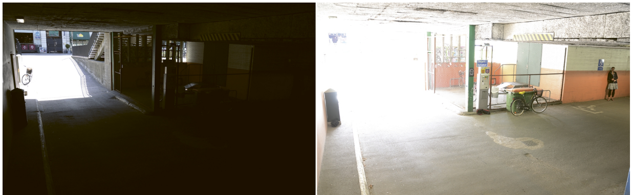
Figure 1. A typical surveillance scene with a wide dynamic range: a parking garage interior with entrance. The two images were taken using different exposure times, shorter for the image to the left, and longer for the image to the right.
