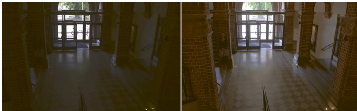
Figure 4. Back-lit interior captured by cameras with different dB values. The image to the right was taken with a camera with a lower specified dB value than the image to the left, contrary to what could be expected.
